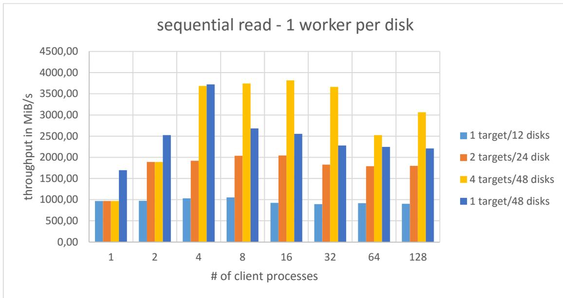
For the tests with 1, 2, and 4 individual RAID6 targets we see that the performance peaks between 8 and 32 processes to a maximum – and reduces a bit when going to 64 and 128 processes due to the higher number of concurrent accesses to the same amount of disk drives
