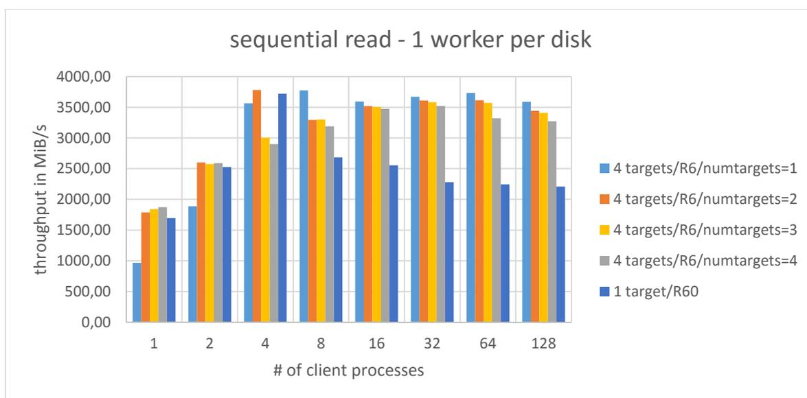
For 1 and 2 client processes any numtargets setting larger than 1 can exceed the performance of the RAID60 target. For 4 client processes a setting of 3 and 4 for numtargets falls behind the RAID60-configuration. For all larger process counts a setting of 1 on the setup with 4 individual targets gives the best result – and the RAID60 configuration is significantly worse.
