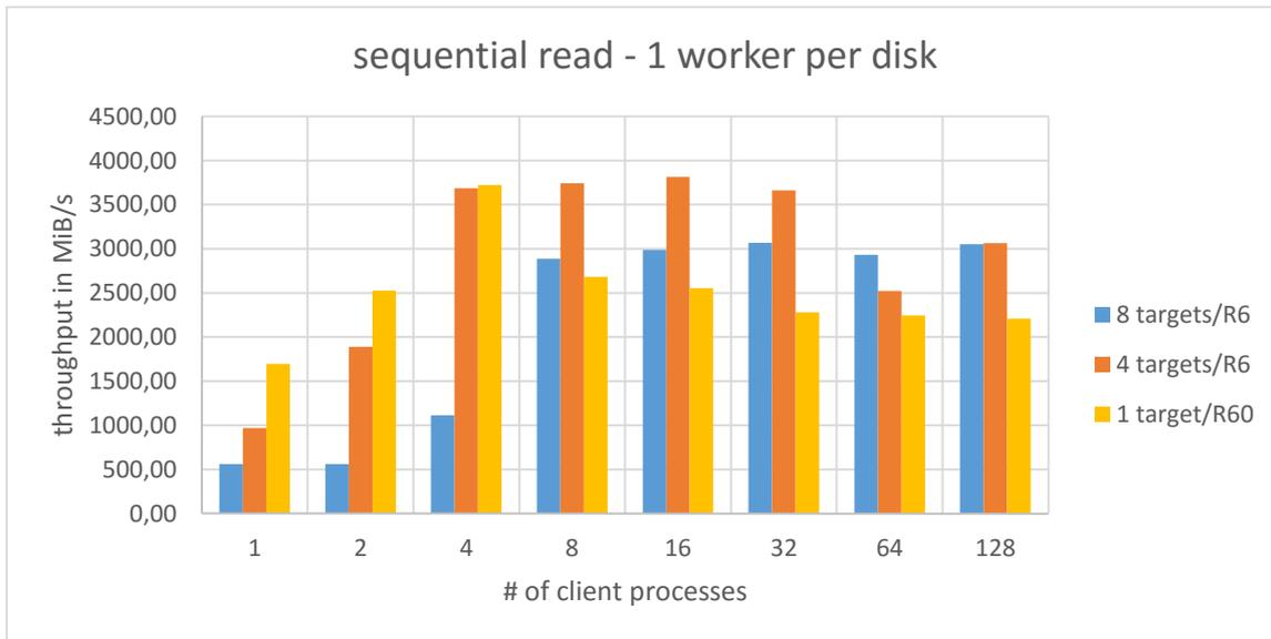
When doing sequential reads we see a significant difference in performance with the 8-target configuration – just for 64 processes we see a slight advantage – and for 128 processes a draw with the 4-target configuration. For all other tests the new configuration performs worse. Especially with a low process count (1, 2, 4) it has a disadvantage as the individual targets are much slower than before.
