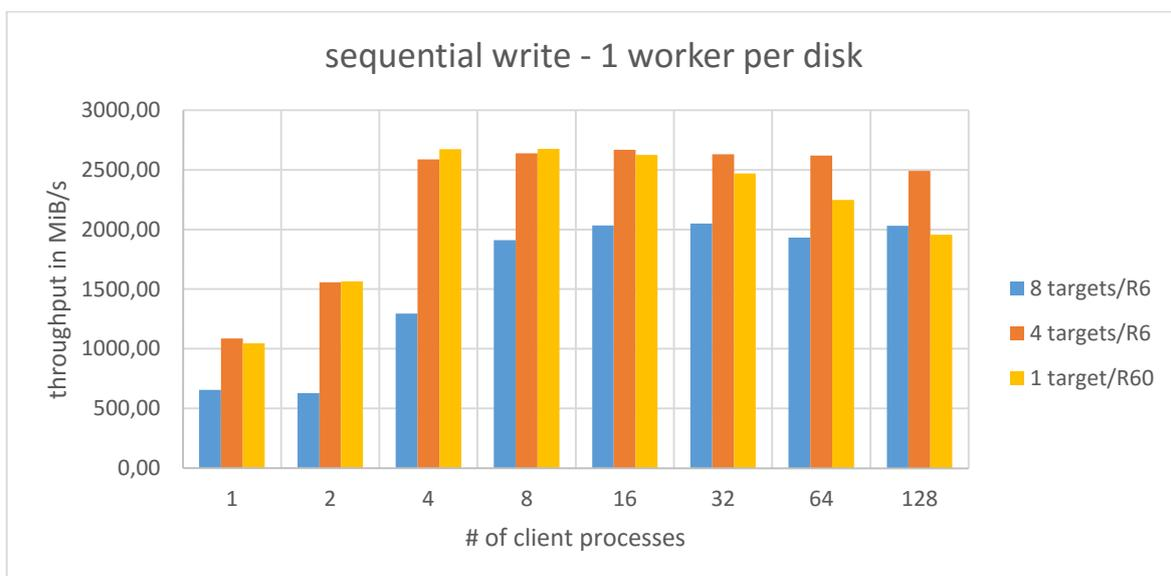
For sequential writes the 8-target configuration performs worse than the 4-target configuration in all tests. This is quite logical when looking at the RAID-mechanism – in a RAID6 4+2 just 4 disks are actually writing user data in a full-stripe where two disks are writing parity data. If the configuration is 10+2 then 10 disks are writing user data.
