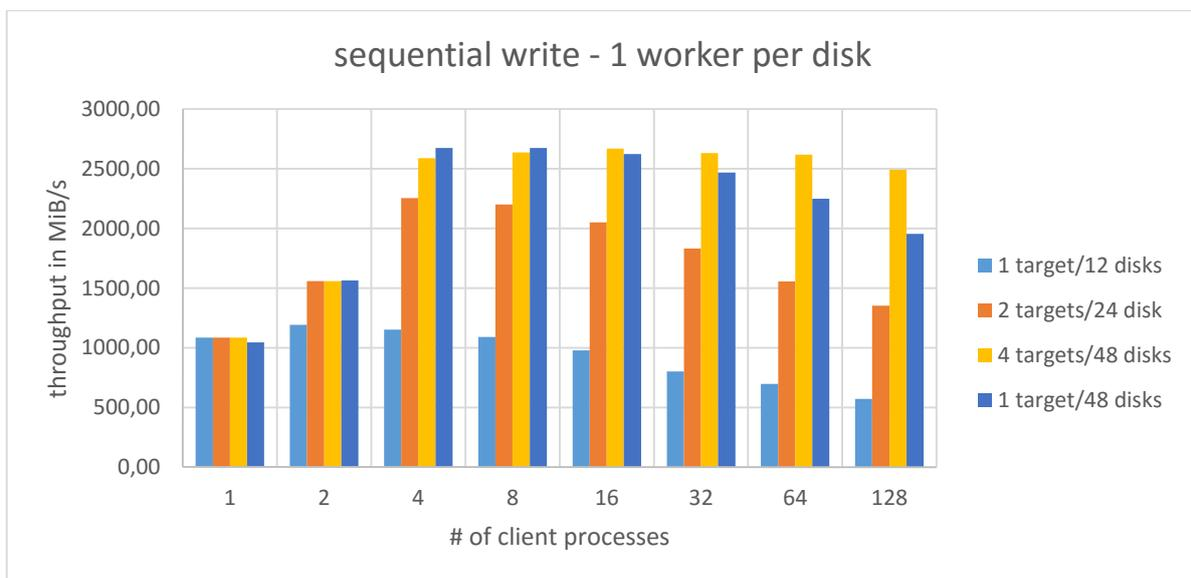
When doing sequential writes the RAID60 configuration has no benefit for lower process counts – but also doesn't lose as much performance as in the read tests when scaling the number of concurrent client processes up. Still it performs significantly worse than the 4 individual targets when 64 and 128 clients are accessing the system.
